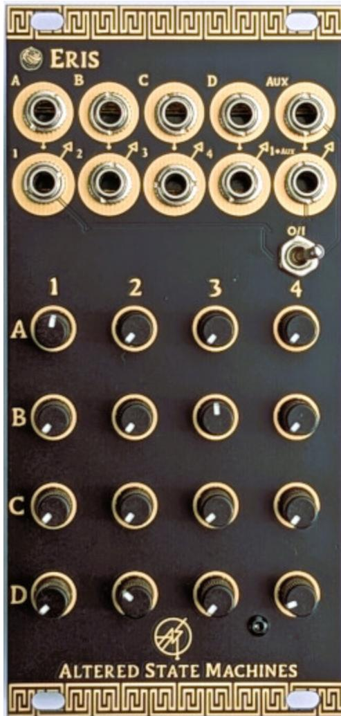
Eris is a four input, four output matrix mixer in 12hp. Each of the four inputs has a potentiometer to send it to any of the four outputs. The module is DC coupled to allow mixing of audio or CV signals, controlled by linear potentiometers. Gain for each channel is up to four times the input signal allowing for make up gain on a low signal, or overdriving a normal signal.
